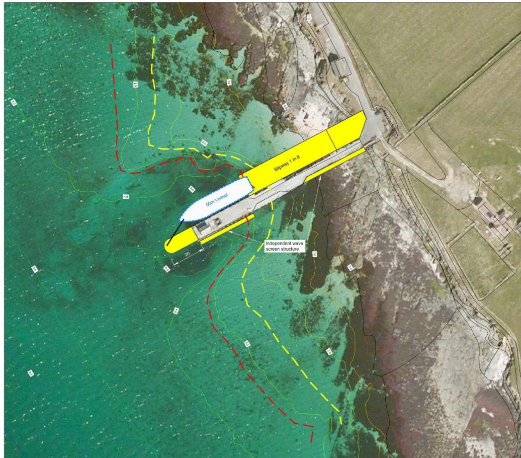
Figure 4.7: Infrastructure Works Required to Accommodate a 50m Slipway Vessel (Vessel Scenario 2)
