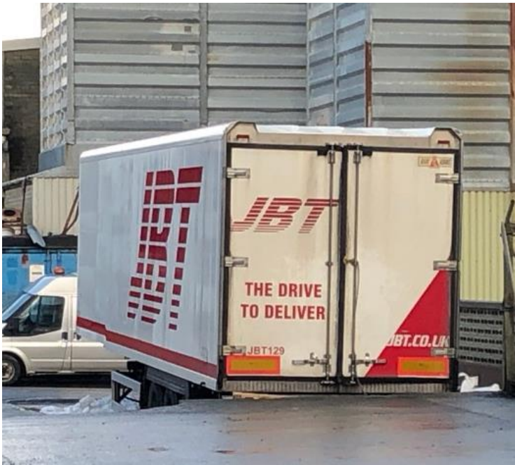
Figure 3.2: Refrigerated trailer used as the temperature controlled holding area (Credit: Martin Bignell, ProVersa)
