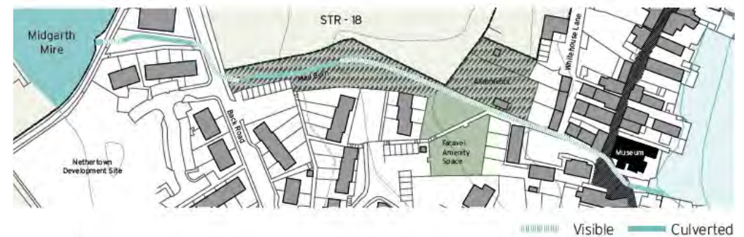
Figure 9: Mayburn Culvert Plan
