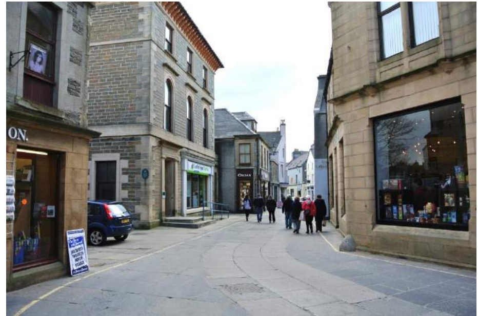
The shared surface of concrete and sandstone flagstones at the junction of Bridge Street and Albert Street
