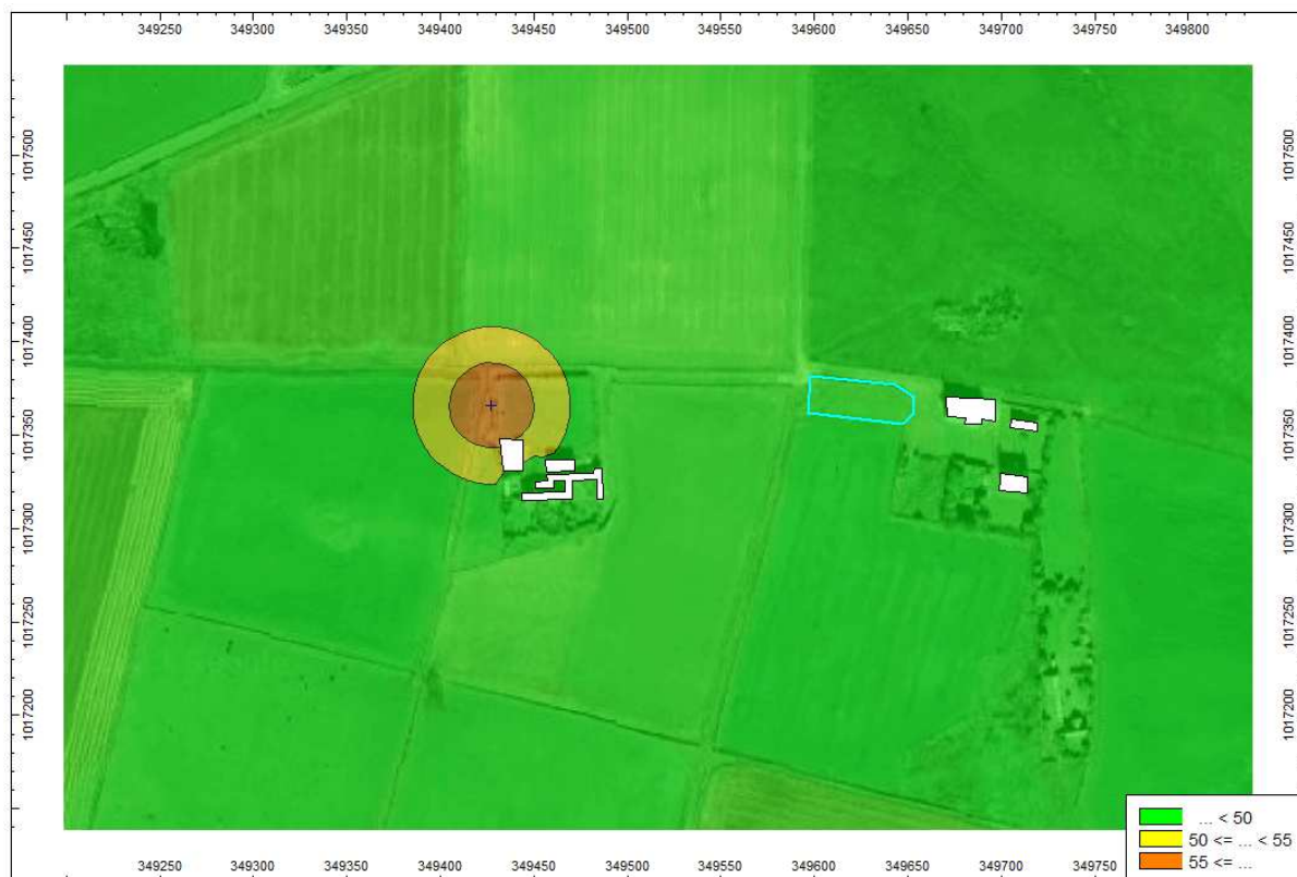
Figure 5.1 Plan view of turbine noise propagation towards proposed development site
