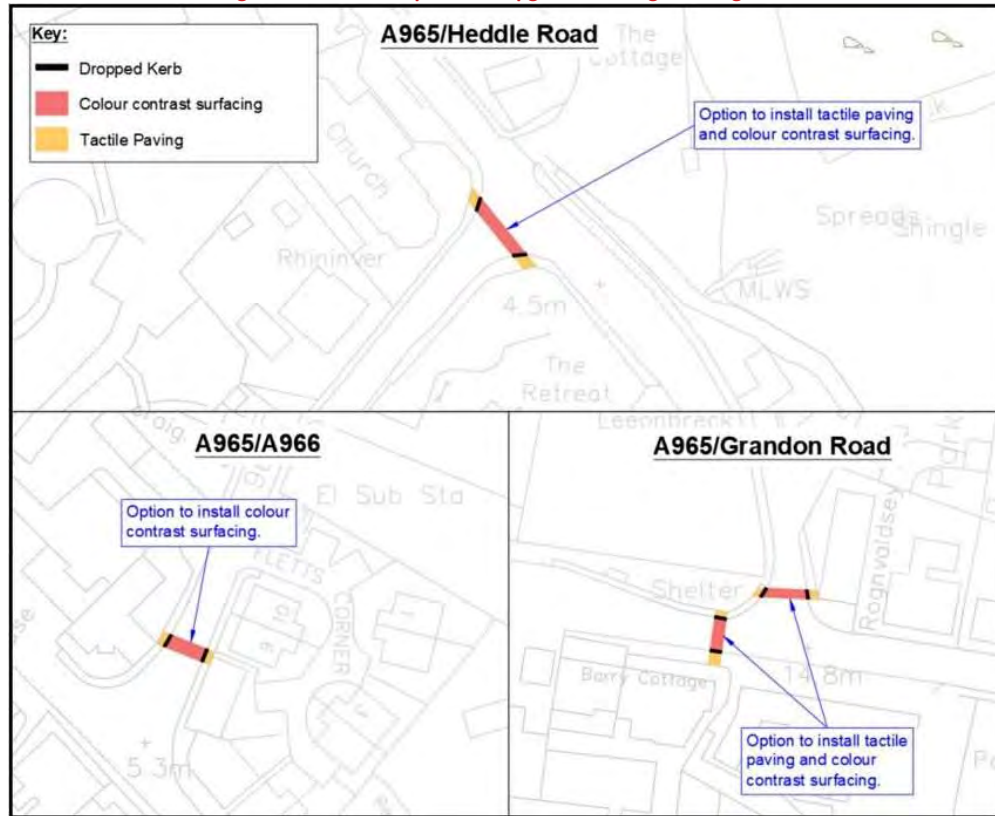
Figure 38. Option 4 – Upgrade Existing Crossing Points
