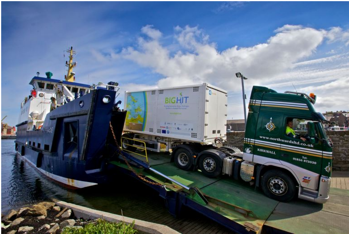
Hydrogen trailer being loaded onto Shapinsay ferry. (Photo credit: Colin Keldie).
